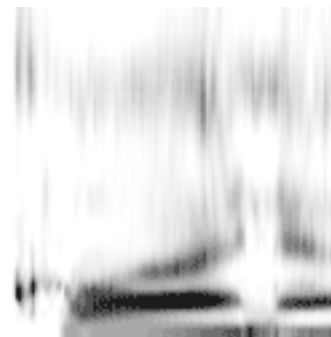
A smooth spectrogram, as shown here, is one step in the audio morphing process.
